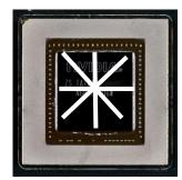
4. PLACING THERMAL PADS ON PCB. Place thermal pads on the circuit board as shown on the picture below. Refer to numbering in previous picture when applying thermal pads of different sizes or thicknesses. EK made sure to provide customers with more than adequate quantity of thermal pads to complete this step.
