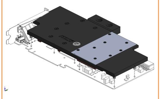
3. ATTACHING THE BLOCK TO THE GRAPHIC CARD. Use a Philips screwdriver screw with the enclosed M3x4 DIN 7985 screws. EKWB recommends users to start tightening the screws around the GPU core and continue outwards. Always use a plastic washer under each and every screw! If the washer is already present on the circuit board (usually around the four GPU core screw holes) there is no need for additional washer.
