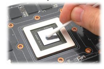
3. APPLYING THERMAL COMPOUND. Wipe off the remains (by using non–abrasive cloth or *q-tip*) of the original thermal compound until the components and circuit board are completely clean. Apply thermal compound: lightly coat *NVIDIA* GPU chip with enclosed EK-TIM Ectotherm thermal grease. EKWB recommends to apply thermal grease in cross form for best performance (see sample picture).
