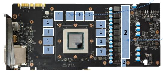
2. PLACING THE BLOCK ON TO THE GRAPHICS CARD. Carefully position the water block with preinstalled 2.5 mm standoffs on to the graphics card. During this process please make sure you align mounting holes on the PCB with holes on the water block (same applies for other tops). Also pay attention not to use too much force by pressing the block down to the PCB. Chip dies are prone to cracking.
