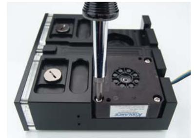
NOTE: If your pump version has feet on the plastic base, these must be removed in order to fit the RP-401X2.
