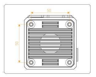
The assembly can be mounted on any flat surface inside your computer chassis. You must drill four (4) 4.2 mm holes using the power drill in a  $50 \times 50$  mm square pattern.
