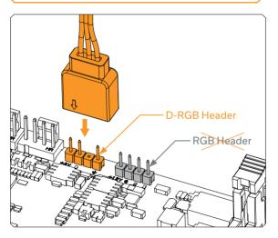
Plug the 3-pin connector from the EK-Quantum Kinetic TBE DDC to the D-RGB header on the motherboard. The LEDs will work if the pin layout on the header is **+5V GRB**.
